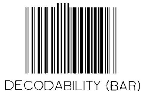
Figure 5.12.5.12-3. Calibration symbol with engineered low decodability grade
